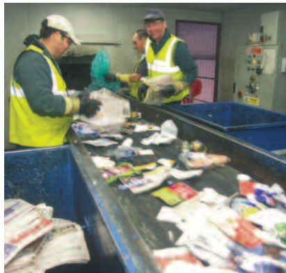
Sorting paper at a Materials Recycling Facility or 'MRF'.
